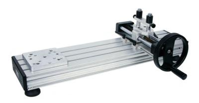
Work with digital torque testers (IST-TT5, IST-TT30, IST-TT50, IST-TT220, IST-TT550)
